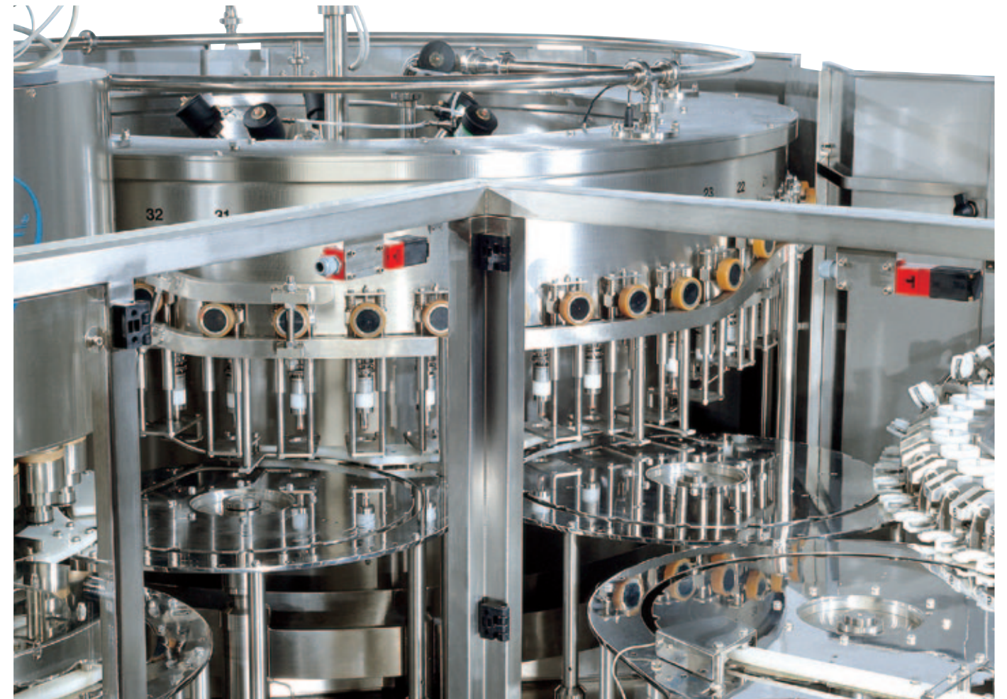
Uniblocco 40/40/8 Particolare: Sistema presa collo Unibloc Model 40/40/8 Incorporating the neck holding system
